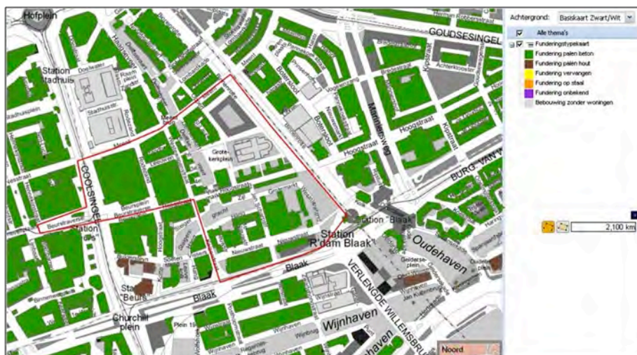
Fig 6.2.2a Centre of Rotterdam, reconstructed after Second World War in green: concrete pile foundations; in brown: wooden pile foundations (historic buildings) Source: Stadsontwikkeling Rotterdam
