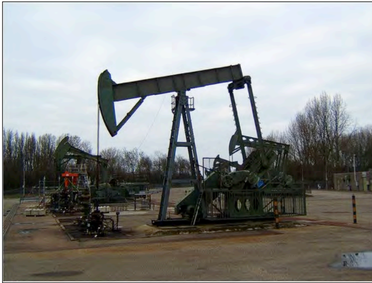
Fig 6.4.1c Nodding donkeys active at Berkel field location until 2013. Oil from the Berkel field was produced from a depth of 1250 metres from the Berkel sandstone reservoirs of the Lower Cretaceous. Source: NAM
