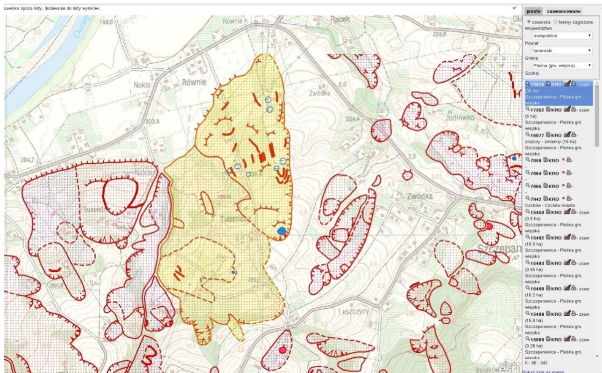
Fig.18. SOPO (Landslide Contraction System) Polish Geological Survey web browser application. An example of landslide inventory. Map presents identified landslides with relation to their Landslide Registration Forms. ( http://geoportal.pgi.gov.pl/portal/page/portal/SOPO/Wyszukaj3 ).
